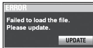
If the above message displays, one or more files necessary for operation of the instrument is missing. You can identify the missing file(s) with MENU - SYSTEM - INFORMATION. The missing file(s) will display “---” instead of a version number.
