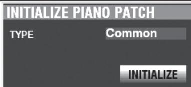
Use the [VALUE] knob to select the Parameters to initialize. Use the DIRECTION [▼] button to move the cursor to the [INITIALIZE] icon and press the [ENTER] button.
