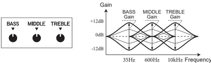
The 3-band Equalizer divides the audio signal into 3 frequency bands (Bass, Middle and Treble) and allows you to boost or cut each band.
