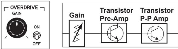
The “Overdrive” effect is a distorted sound created by routing the audio signal into the transistorized “Push-Pull” amplifier.
