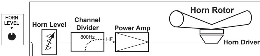
Use this control to adjust the level of the Horn Driver and to balance the sound between the Horn Driver and Woofer.
