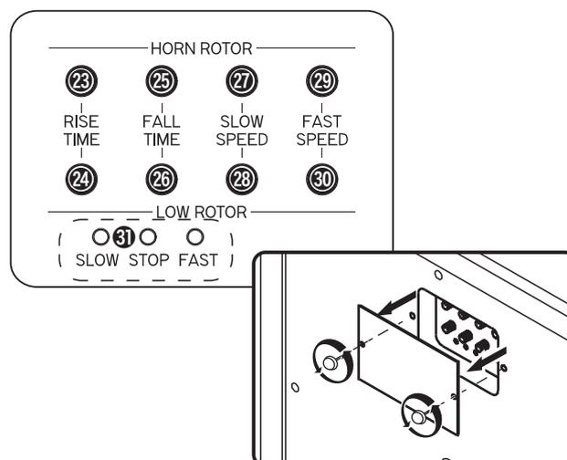
The Rotor Control Panel is located inside the ornamental Nameplate on the back panel of the cabinet.\*
