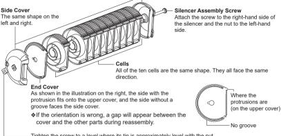
Tighten the screw to a level where its tip is approximately level with the nut.
