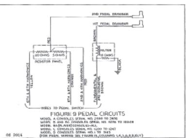
FIGURE 9 PEDAL CIRCUITS
