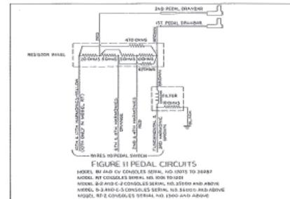
FIGURE 11 PEDAL CIRCUITS
