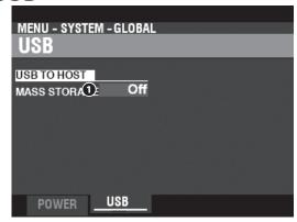
This allows you to Load and Save files from the instrument's Internal Memory and access files to or from a host computer via a USB cable.
