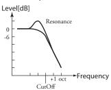
LP12/LP24...... Low-Pass 12(24)dB; reduces above the Cutoff Frequency at 12(24)dB/octave.
