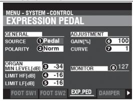
This Page allows you to control how a connected Expression Pedal will function.
