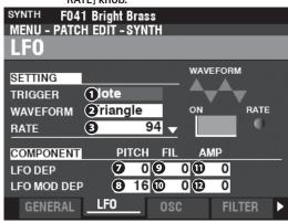
This Page allows you to adjust the "Low Frequency Oscillator" (LFO, which creates Vibrato or Tremolo effects) and its depth.
