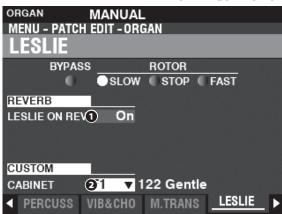
This Page allows you to adjust the Parameters affecting the inbuilt digital Leslie for the Tone Wheel and Transistor Organs.
