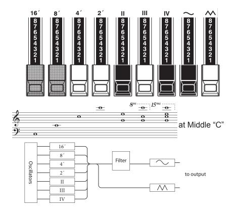
The type of British combo organ replicated by the "Vx" ORGAN Type had Drawbartype controls, but they functioned differently from Hammond Harmonic Drawbars. The first four Drawbars control individual pitches, while the next three are "Mixture" Drawbars which cause multiple pitches to sound. "II," "III" and "IV" refer to the number of pitches represented by that Drawbar.
