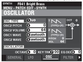
This Page allows you to adjust the oscillating method or pitch.
