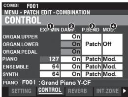
This Page allows you to select which Parameters of each Voice Section will be Recorded as part of a Combination.
