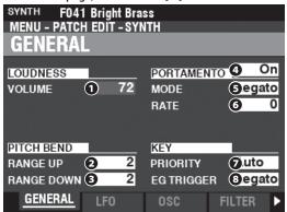
This Page allows you to adjust the common Parameters of a MONO SYNTH Patch.
