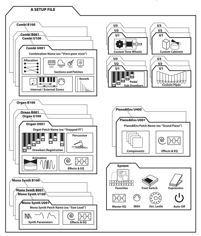
This FUNCTION Mode allows you to save contents in the SKX PRO to a USB Flash Drive or Internal Memory.
