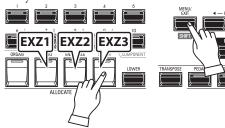
You can allocate External Zones by Press and Hold the [SHIFT] button and pressing [PIANO] for External Zone 1, [ENSEMBLE] for External Zone 2 or [SYNTH] for External Zone 3 (see the illustration above).
