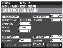
This Page allows you to adjust the Parameters which affect the Virtual Multi-Contacts and the Sustain effect for the UPPER and LOWER Parts.
