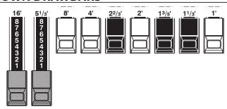
The two brown Drawbars on the far left give depth and richness to the sound. The left 16' is one octave lower than the 8', and 51/3' is the third harmonic of the 16' fundamental. Normally, the tones are built on the 8' fundamental, but, if you want to add depth to the tone or to expand the playing range by one octave lower, build your tones on the 16' fundamental.
