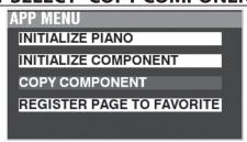
Use the DIRECTION [▼] button to move the cursor to "COPY COMPONENT" and press the [ENTER] button.
