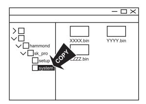
Copy the ".bin" update files into the "system" sub-folder of the USB Flash drive or the Internal Memory.
