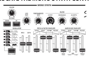
Use the controls in the MONO SYNTH portion of the Control Panel to create a MONO SYNTH Patch.
