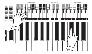
The Drawbars control the basic organ sounds. You can hear the effect each Drawbar has on the sound by pulling out or pushing in Drawbars while holding keys.
