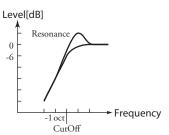
HP12/HP24..... High-Pass 12(24)dB; reduces below the Cutoff Frequency at 12(24)dB/octave.
