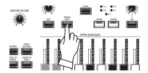
The ORGAN Section has 3 Parts - UPPER, LOWER and PEDAL. The [ORGAN SOLO] button turns all the Parts of the Organ Section "ON," and turns other Sections "OFF." This allows you to turn the SKX PRO into a vintage 2-keyboards-and-pedal Hammond Organ instantly with one button press.
