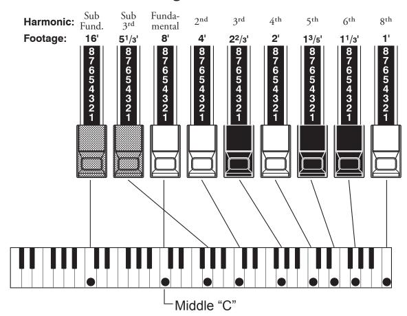
Each Drawbar may be set in eight different positions in addition to the silent or "0" position. Each position, as marked on the Drawbars, represents a different degree of intensity of the harmonic it controls. When drawn out to position "1," the harmonic it represents will be present with minimum intensity, when drawn out to position 2 with greater intensity, and so on up to position "8."
