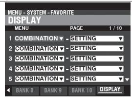
This page allows you to associate and confirm the assignment of display pages to numbered buttons.
