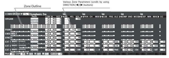
The Internal Zones and the External Zones are advanced features for controlling internal sound engine or external MIDI equipment. See "Combination" of the page 74 for details.
