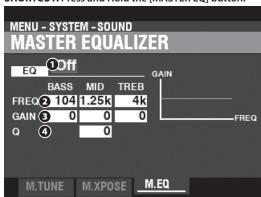
This Page allows you to adjust the overall tonal quality of the instrument.
