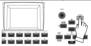
After you have made your changes to SYSTEM Parameters, press the red [RECORD] button. The RECORD Page will display.
