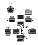
Use the DIRECTION buttons to move the cursor to the Parameter you wish to adjust. For this example, select "DECAY FAST."
