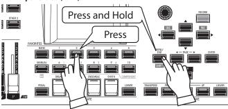
To locate an associated display page, Press and Hold the [SHIFT] button and press a numbered [FAVORITE] button.
