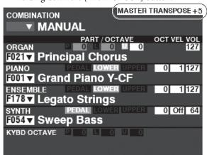
In the above example, the TRANSPOSE value is set at "+5" - if a "C" key is depressed, a note five (5) half-steps higher will sound ("F").
