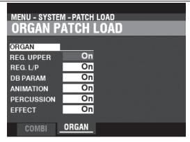
This Page allows you to select which Parameters to include as part of an ORGAN Patch.
