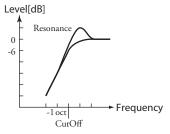
**HP12**.....High-Pass 12dB; It reduces under Cutoff Frequency at 12dB/octave.
