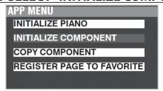
Use the DIRECTION [▼] button to move the cursor to [INITIALIZE COMPONENT] and press the [ENTER] button.
