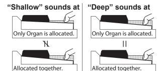
NOTE: If "Shallow" is selected and a key is depressed, the ORGAN Section will sound when the key travel reaches the "Shallow" sounding point, but MIDI Note data will not be transmitted unless or until the key reaches the "Deep" sounding point. If the key reaches the "Shallow" sounding point but does not travel all the way down to the "Deep" sounding point, MIDI Note data will not be transmitted.
