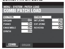
This Page allows you to select which Parameters to include as part of a Combination.
