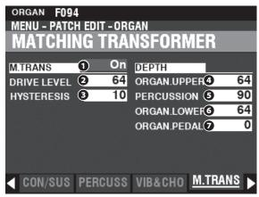
This Page allows you to adjust the Parameters affecting the Matching Transformer for the Tone Wheel and Transistor Organs.
