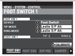
This Page allows you to select the Function of devices connected to the Foot Switch [FOOT SWITCH 1/2] jacks.
