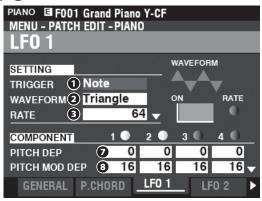
Both the PIANO and ENSEMBLE Voices Sections have two LFOs (Low Frequency Oscillators). These can be used to modulate various Components or Parameters.
