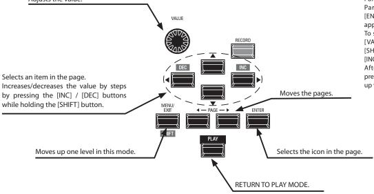
[ENTER] button. A pop-up screen will appear showing the available options. To select the option you wish, turn the [VALUE] knob or Press and Hold the [SHIFT] button and press the [DEC] or [INC] buttons.
