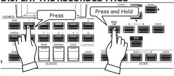
To display the Recorded Page, Press and Hold the [SHIFT] button and press the numbered [FAVORITE] button.
