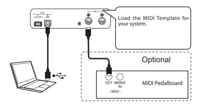
To control a MIDI Sound Module from the SKX PRO using both a single keyboard and Expanded Keyboards, do the following:
