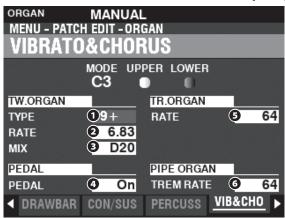
This Page allows you to adjust the Vibrato & Chorus of the Tone Wheel Organs, Vibrato for the Transistor Organs, and Tremulant for the Pipe Organ.
