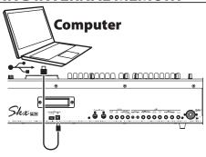
Connect the [TO HOST] port and the computer via USB cable.
