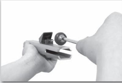
Tighten head mounting screw with a screwdriver(No.2) sold separately.
